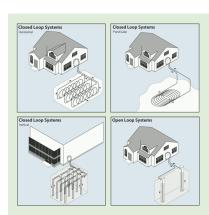
Figure 2: Closed-and open-loop geothermal heat pump systems. Source: http://energy.gov/ energysaver/geothermalheat p
